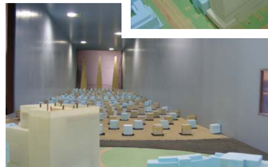
Model of research facility tested in a wind tunnel. Emissions are modelled to represent actual momentum and buoyancy of the full-scale stacks.
