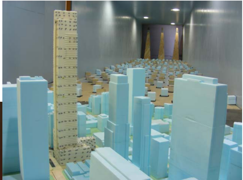
Photograph showing scale model of a study building in its urban surrounding installed in GmE's wind tunnel
