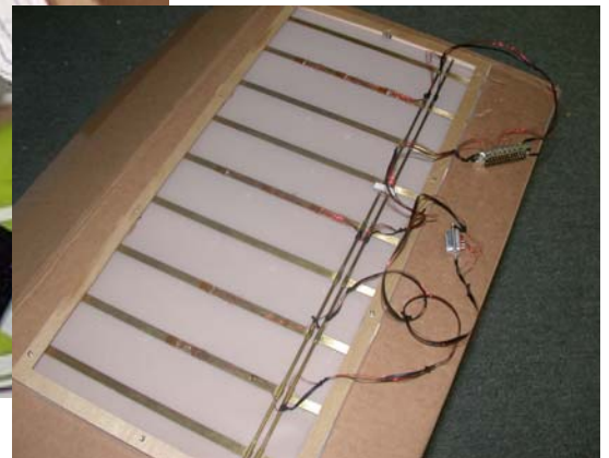
Strain Gauges Are Used to Obtain Peak Wind Loads On The Simulated Roof Members
