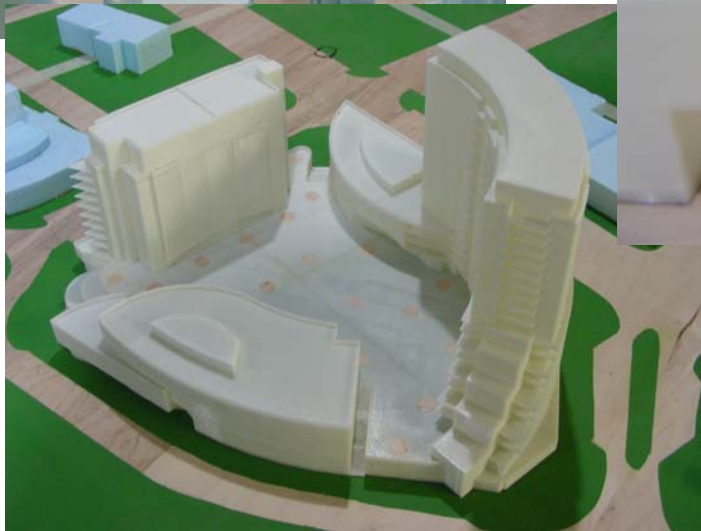
Pedestrian level wind sensors on podium of future building planned for an urban area.
