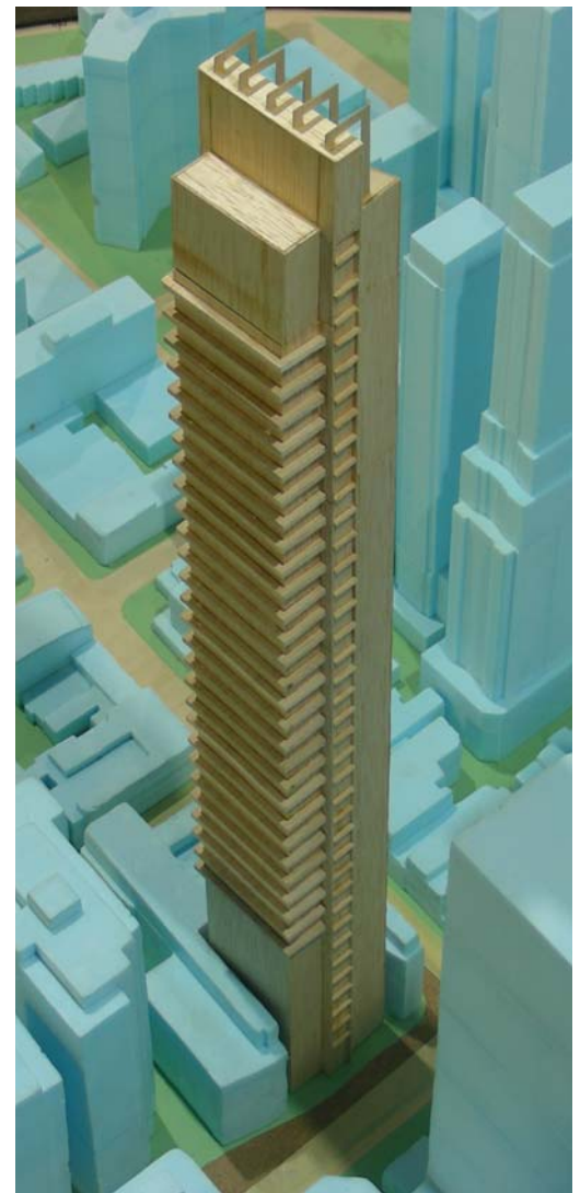
Light Weight Building Model Installed On HFFB Base
