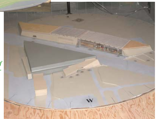
Aeroelastic Model of Long Span Roof For Aircraft Hangar
