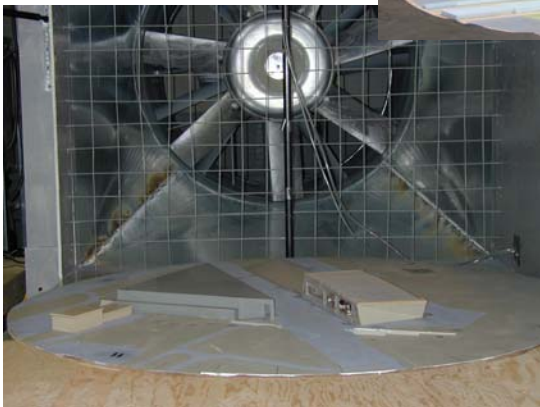
Aeroelastic Model of Long Span Roof For Aircraft Hangar
